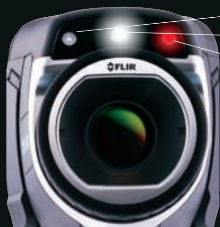
Visible Light Pictures Align with Thermal Images
